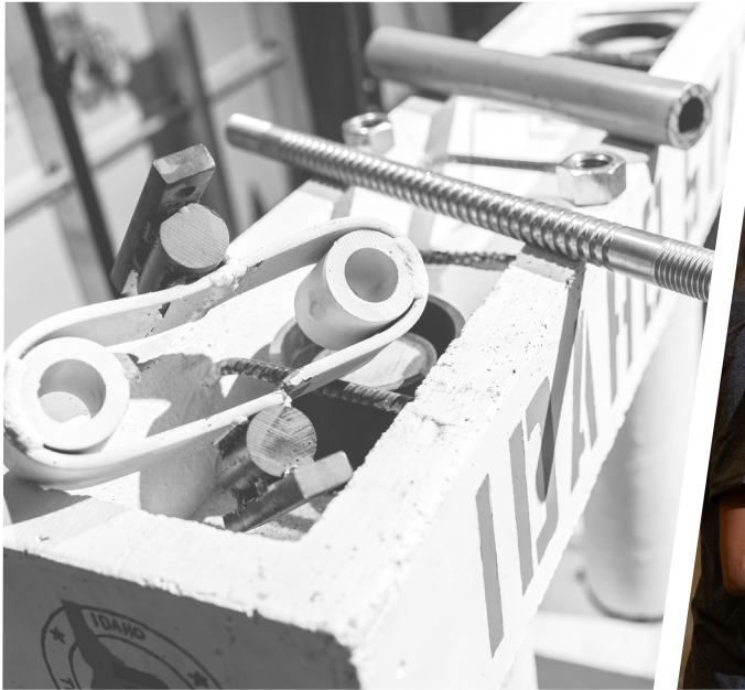
Left: Metal dissipators used in the ISU Structural Laboratory. Right: Mustafa Mashal, Ph.D., Associate Professor (right), leads the Structural Laboratory.
